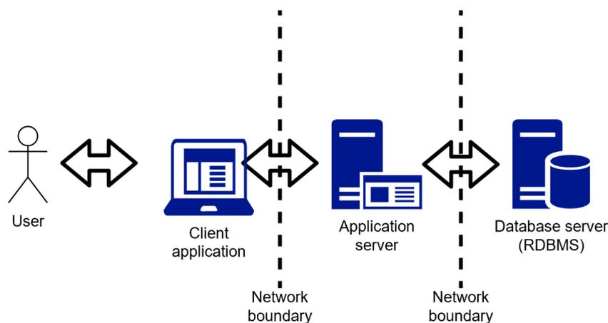
Figure 1: Basic interactions between the user and the database server
