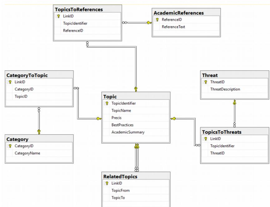
Figure 5.1: UML entity-relationship diagram for the DSF schema
